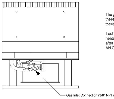
The gas inlet connection is 3/8" NPT, made at the rear of the main control through the area at the rear of the pedestal.
